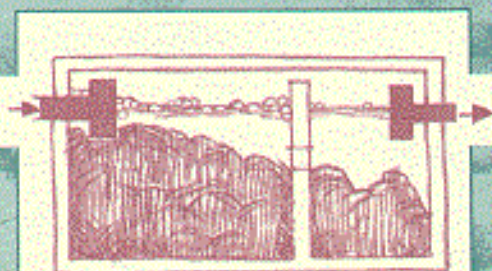
A cross-section shows settled solids and floating scum decreasing the tank's available capacity.
